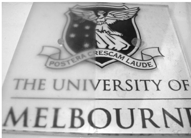
Fig. 1: Two views of the same glass plate where the slightly opaque half has been made into a silica nanoparticle super hydrophobic surface. The clear half is uncoated glass. The drops of water, tinted in red, have a high contact angle on the super hydrophobic side but spreads on the uncoated side.
