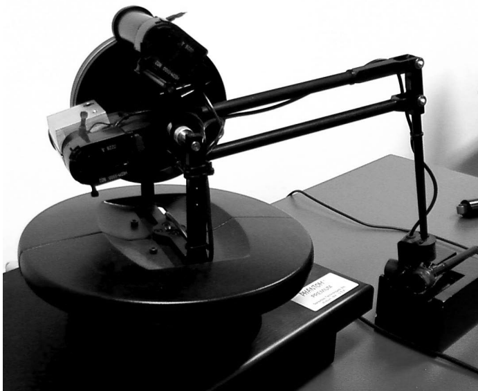
Fig. 1. Phantom 1.5 Haptic Probe from SensAble Technologies.
